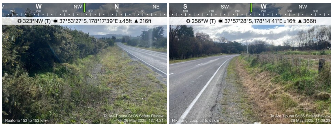
Figure 2.1-5: Typical shoulder width constraints
